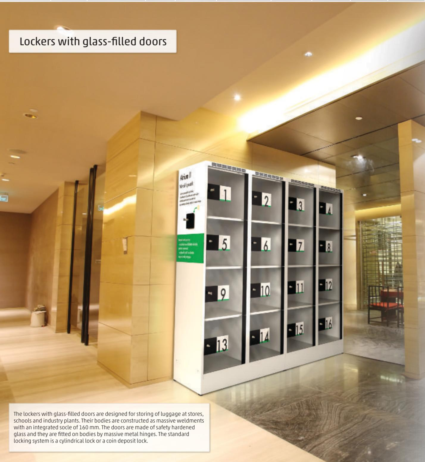
The lockers with glass-filled doors are designed for storing of luggage at stores, schools and industry plants. Their bodies are constructed as massive weldments with an integrated socle of 160 mm. The doors are made of safety hardened glass and they are fitted on bodies by massive metal hinges. The standard locking system is a cylindrical lock or a coin deposit lock.
