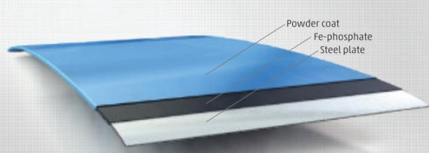
The input material is steel plate or steel profiles. In painting line IDEAL-LINE there is applied a Fe-phosphate layer and the segments are dried. It ensures a better adhesion of the powder coat to the base coat. The powder coat of the desired shade is then applied onto the segments in electrostatic field and then it is hardened at temperature of approx. 180 °C. The final coat is hygienic, flexible and scratch resistant.
