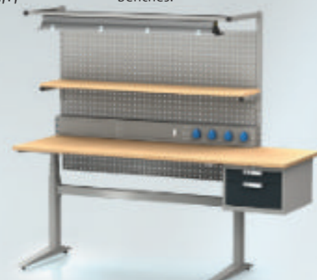
Order code Width (mm) Price (€) alnak 15 K05 2000 3347,9,- Width of upper extension is 1500 mm, beams 20U H903 mm with assembly slots, spacing 22 mm, back covering sheet, 3x EUROPERFO® panel 5U, shelf 300 mm, energy channel K1, illuminating body holder, lamp ALMAX, cabinet DKU 6U 2AS.
